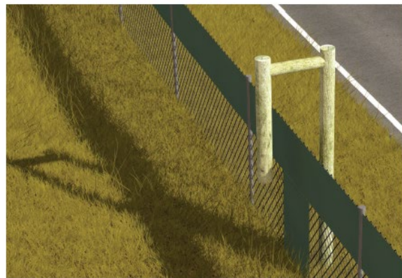
Figure H4 Escape pole with an alternative design to the H-shaped escape pole
